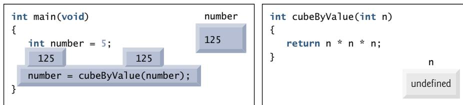
Fig. 7.8 | Analysis of a typical pass-by-value.
