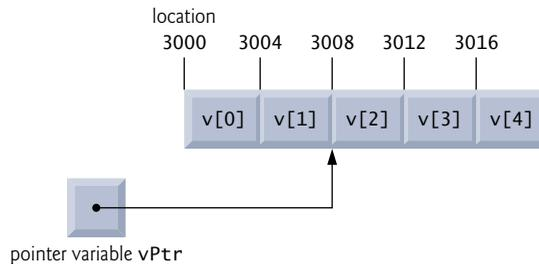
**Fig. 7.19** | The pointer `vPtr` after pointer arithmetic.
