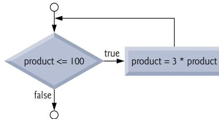
**Fig. 3.4** | Flowcharting the `while` iteration statement.
