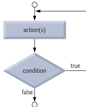
**Fig. 4.10** | Flowcharting the `do...while` iteration statement.
