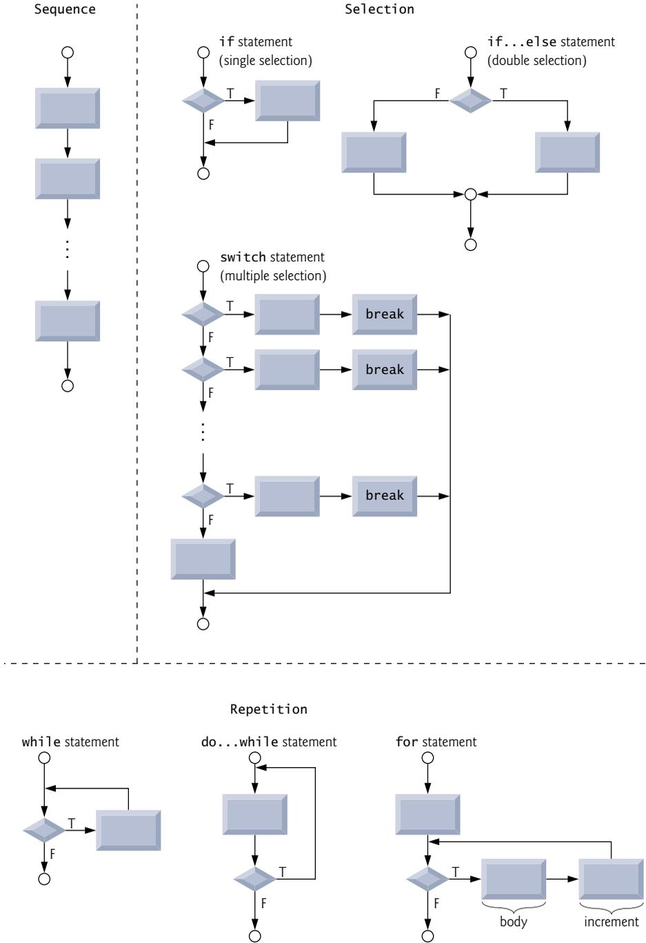
**Fig. 4.17** | C's single-entry/single-exit sequence, selection and iteration statements.
