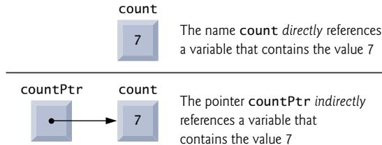
**Fig. 7.1** | Directly and indirectly referencing a variable.
