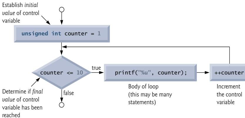
**Fig. 4.4** | Flowcharting a typical for iteration statement.
